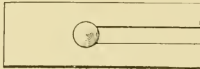
Fig. 238—A hole drilled at the end of the cut will automatically remove the chip
